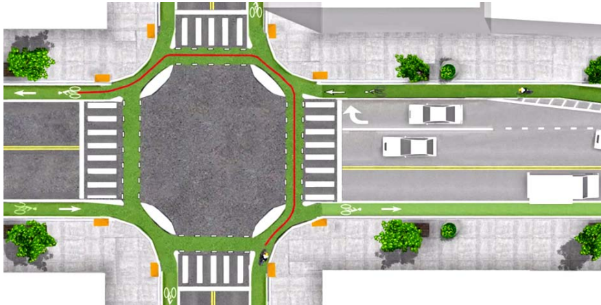
(Above): This design minimizes conflict points between vehicles and bicyclists. A bicycle rider, by using the green lane, is able to make a left turn in one fluid motion, without going through the middle of the intersection. At the island areas, they have refuge points.
